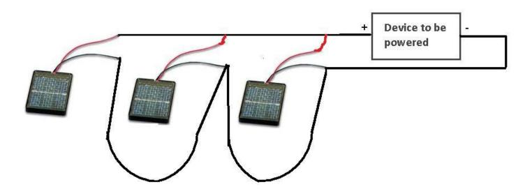
When you connect solar cells in parallel, the current of each cell adds up. You increase the net current of the circuit. For example, if you tie 3 solar cells together and each has a current rating of up to 0.1A in bright light, the net current will be 0.3A, or 300mA, since the 3 currents add together. In parallel, currents add. Voltage stays the same. So if each solar cell had a voltage rating of 0.5V, the circuit will output 0.5V.
