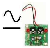
In this project, we will build a device that can indicate to us whether the voltage flowing through it is AC or DC, and for DC, it can tell whether the current is flowing forward or flowing in reverse.
