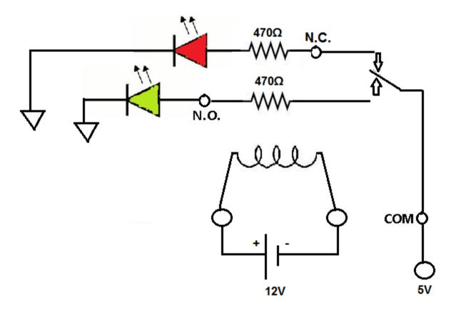
The SPDT relay that you get most likely will be one which operates on 12V. This means that you must feed the coil of the relay 12V in order for it to operate and function.
