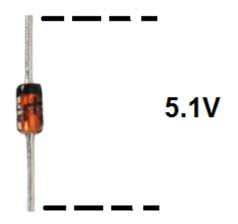
A Zener Diode is a special type of diode that is used most extensively as a voltage regulator; this is because once the reverse voltage supplied to a zener diode reaches its breakdown voltage, referred to as Vz, the voltage across the diode remains very constant at this voltage even if the current through the diode continues to increase or vary.
