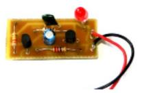
In this project, we will configure a circuit that causes an LED to flash.
