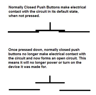
When the button is pressed down, the switch no longer makes electrical contact and the circuit is now open. Therefore, electricity can no longer flow to the other part of the circuit to turn or power on the respective part of the circuit the button was made to switch.
