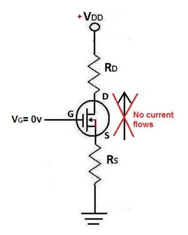
However, if a voltage is applied to the gate lead of the MOSFET, the drain-source channel becomes less resistive. As the gate voltage increases more and more, the current flowing from source to the drain increases more and more, until maximum current is flowing from source to drain.
