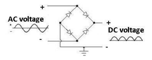
A full wave rectifier takes an AC signal input into it, such as the AC signal from a power outlet, and converts it into a DC signal. The AC is input. The DC is output.
