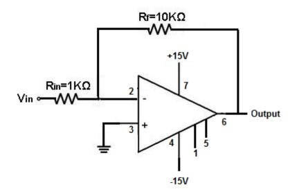
At V<sub>in</sub> of the schematic diagram above, we input the input AC signal which we want to amplify. We connect the positive part to the inverting pin of the op amp and the negative part into ground. And the output pin is where we retrieve our amplified output signal.
