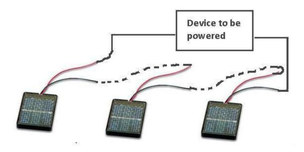
When you connect solar cells in series, the voltage of each cell adds up. You increase the net voltage of the circuit. For example, if you tie 3 solar cells together and each has a voltage rating of up to 0.5V, the net voltage will be 1.5V, since the 3 voltages add together.
