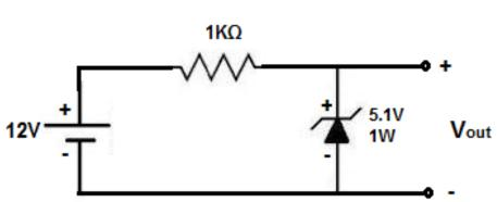
Zener Diode Voltage Regulator Circuit
