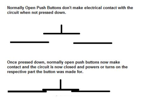
When the button is pressed down, the switch makes electrical contact and the circuit is now closed. Therefore, electricity can now flow to the other part of the circuit connecting to the push button and make the device turn or power on the respective part.
