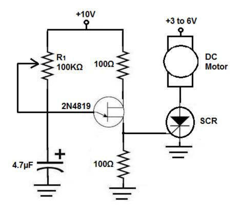
The  $100\Omega$  resistors are just to bias the UJT transistor. They are small resistors to help limit current passing through the base leads of the UJT.
