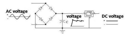
You can see after the smoothing capacitor that the voltage is pretty steady but not quite. After the voltage regulator, it should be nearly perfectly steady and even. This will produce the most precise DC voltage. A voltage regulator is a device that regulates a specific DC voltage output. It has 3 terminals, an input terminal, an output terminal, and ground. The input terminal receives the voltage that a user wants to regulate down. The
