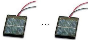
In this project, we will build a battery recharger from solar cells. Solar cells, which harvest energy from light, convert the light energy into electrical current, which then charges a battery or batteries. In this project, you'll learn how solar cells can be connected to give enough power output to recharge a rechargeable battery.
