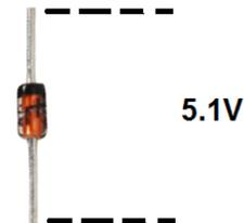
In this project, we will show how to connect a zener diode in a circuit to act as a voltage-regulating device, which is a device that outputs a constant DC voltage across its terminals. You will learn what zener diodes are, their characteristics, and how they can be connected in a circuit to provide a constant, stable voltage to any device we want to feed.
